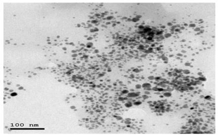
Figure 2. shows TEM image of silver nanoparticles which revealed the average size of silver nanoparticles.
