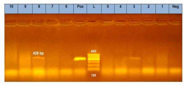
Lane L: Molecular marker; Lane pos: Positive control; Lane Neg: Negative control; Lanes 1,2,4-7,9,10: negative for Plantaricin E/F; Lane 3,8: positive isolates for Plantaricin E/F.
